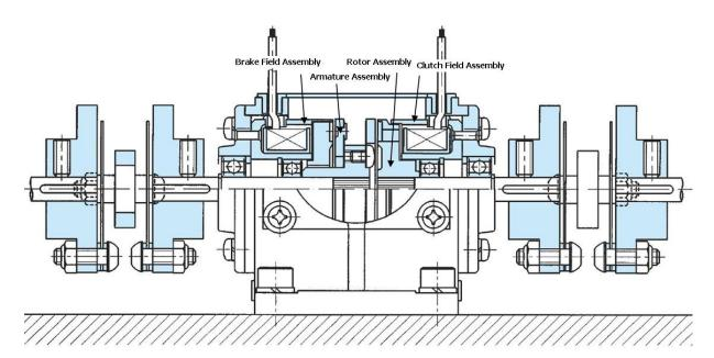
The mounting surface should be made flat by machining. When couplings are used, care should be taken to the shaft alignment.
