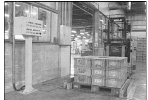
Automated vehicle picking up inbound parts to deliver to the assembly line
