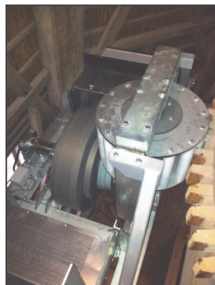
Windmill wooden drive gear driving new plastic roller gears and clutch/generator
