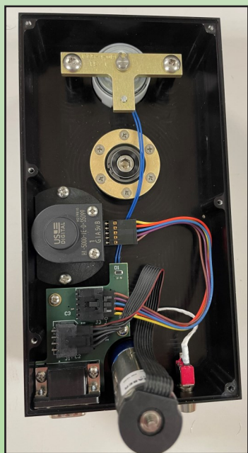
Ogura's MIC-3.5T clutch used as a power-on brake
