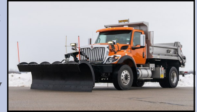
Municipal snowplows can use a front-mount PTO to run power-hungry hydraulic accessories
