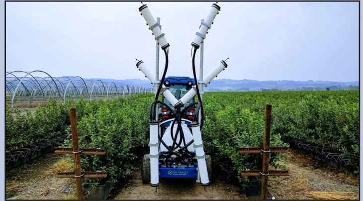
OnTarget sprayer with Ogura blower
