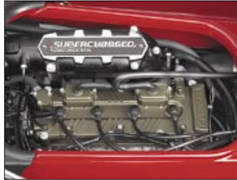
The Ogura Supercharger is custom built into the Kawasaki engine
