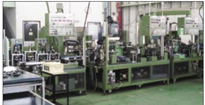
Final combined armature assembly layout
