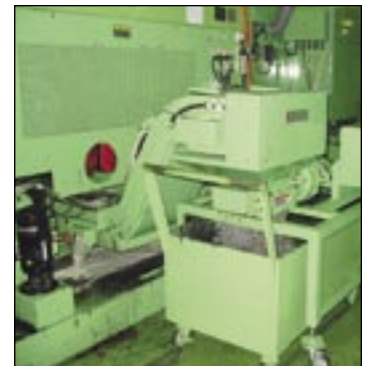
New chip crusher
