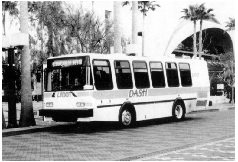
Bus with microturbine hybrid-electric drive system
