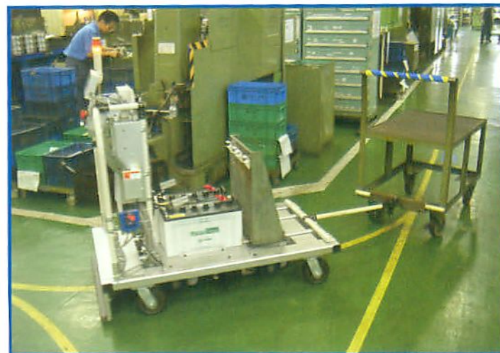
Ogura in-house designed Automated Guided Vehicle with pull cart
