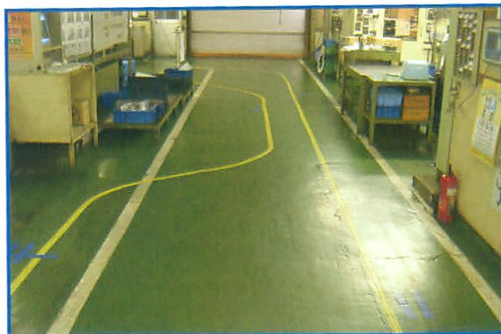
Magnetic Tape applied to the Production floor
