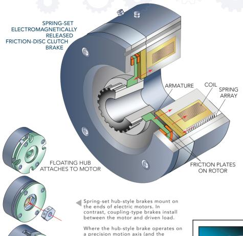
In power-off friction brakes, spring pressure forces the friction discs (or elements) into engagement to stop and hold the load. Then an electromagnetic or pneumatic release system spreads the elements apart to disengaging the unit. Such spring engagement offer a key advantage — the ability to serve as failsafe brakes even during power loss. That contrasts with the electromagnetically engaged brakes.
