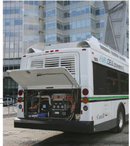
Figure 2 Ogura TX04U-MA is installed in the FCvelocity®-HD6 module, which is located in the Bus engine bay
