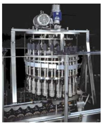
On the capping machines at U.S. Bottlers Machinery Co., the chuck, on a shaft attached to a clutch, picks up the cap. A bottle remains stationary under the chuck as it turns in the correct direction to screw on the cap. It's the job of the clutch to make sure the machine tightens the cap just the right amount.
