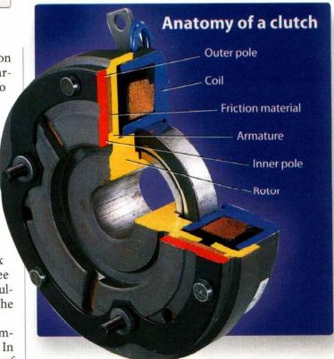
In an EM clutch, current running through the coil generates a magnetic field that attracts the armature toward the rotor. The rotor connects via a hub to the rotating input, like a driveshaft, while the armature connects to the output. Contact transfers torque between the armature and rotor, bringing the output up to the input speed.
