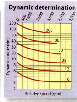
Designers can use manufacturergenerated curves to determine dynamic torque at a given rpm from a clutch or brake's static torque rating. **Each curve** represents a different static rating.
