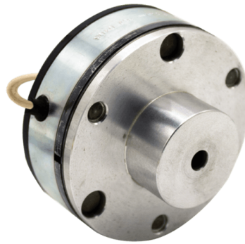
Permanent magnet brakes, like the one shown here, use independent permanent magnets to counteract and oppose the magnet flux generated when power is supplied to the coil of the brake. Ogura Industrial Corp.
