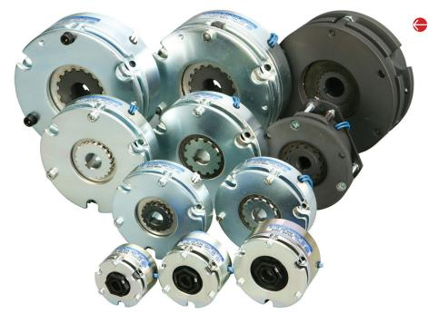
and pressure plate. When applying current to the brake coil, it generates electromagnetic flux to travel across that airgap, which then pulls the pressure plate against the coil body. This compresses the springs that supply the normal force for the brake torque. The brake is then free to rotate.
