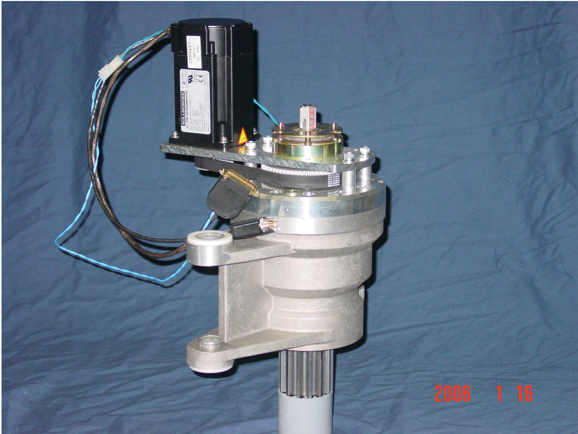
View of the Ogura SNB-0.2G brake on the back of the drive module.
