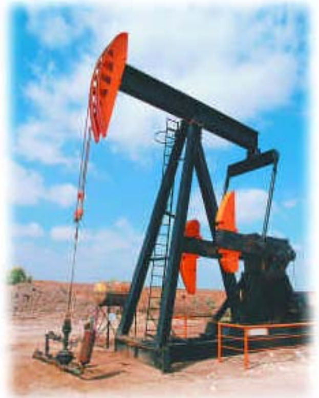
Pumpjack with natural gas engine
