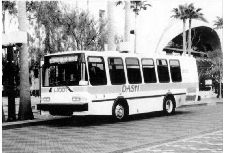
*Bus with microturbine hybrid-electric drive system*
