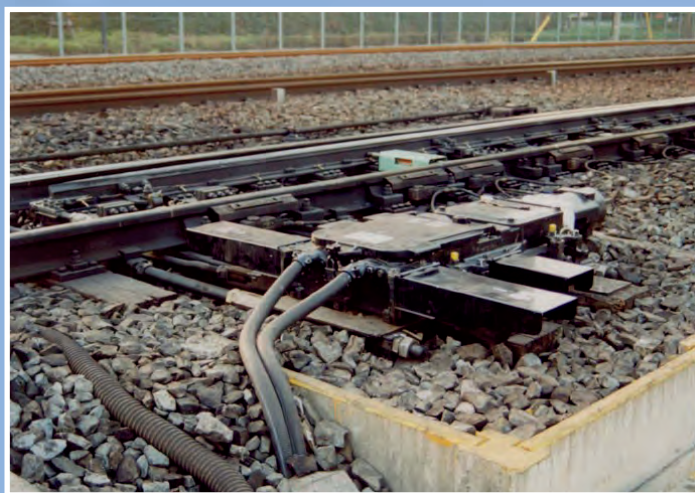
Railroad track switch with PHT 125
