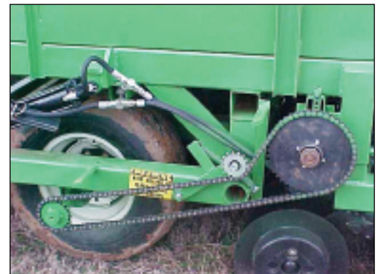
Wheel (ground) driving clutch
