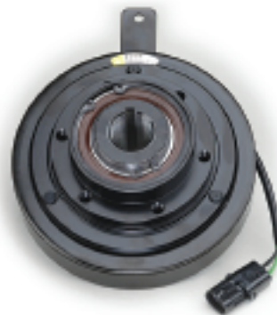
Clutch before sprocket is attached
