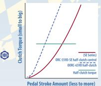
**Drivetrain Protection:** By increasing the half-clutch area, we have reduced the impact torque when the clutch is engaged during a shift change.
