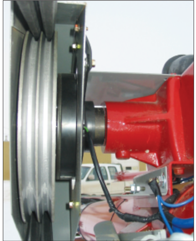
Auger input with pulley mounted to Ogura clutch
