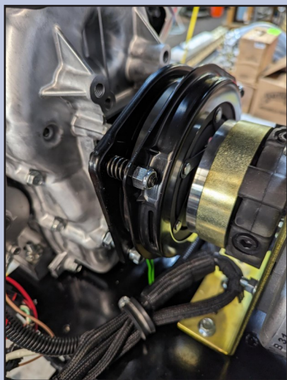
Ogura's GT3.5 clutch with direct mount coupling
