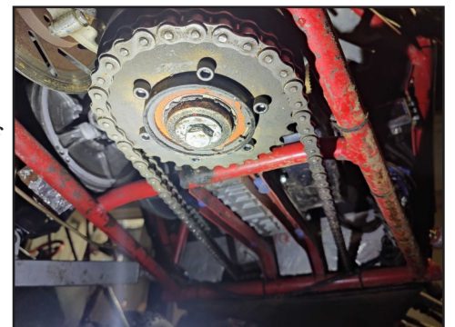
Ogura clutch used to engage front wheel drive via chain
