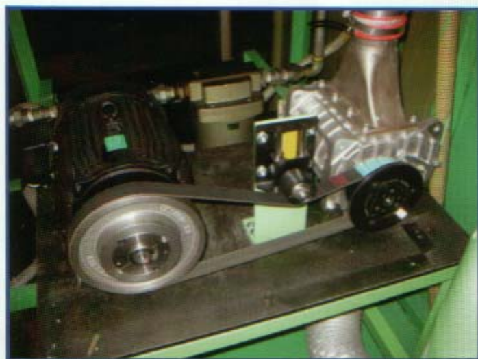
New high efficiency IPM motor and Ogura Air Pump replaces compressor system, saving money and helping the environment
