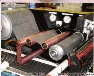
goes through a load cell that measures wire tension as it is pulled into a wire twister. The load cell feeds back tension information to the controller, which in turn feeds voltage back to the brake. Voltage is proportional to torque (assuming a constant current power supply) in magnetic particle brakes, so this provides relatively simple tension control.
