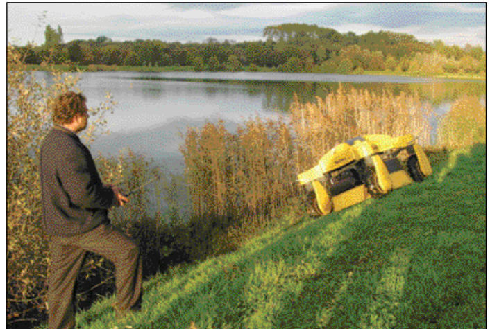
Mower being controlled with remote
