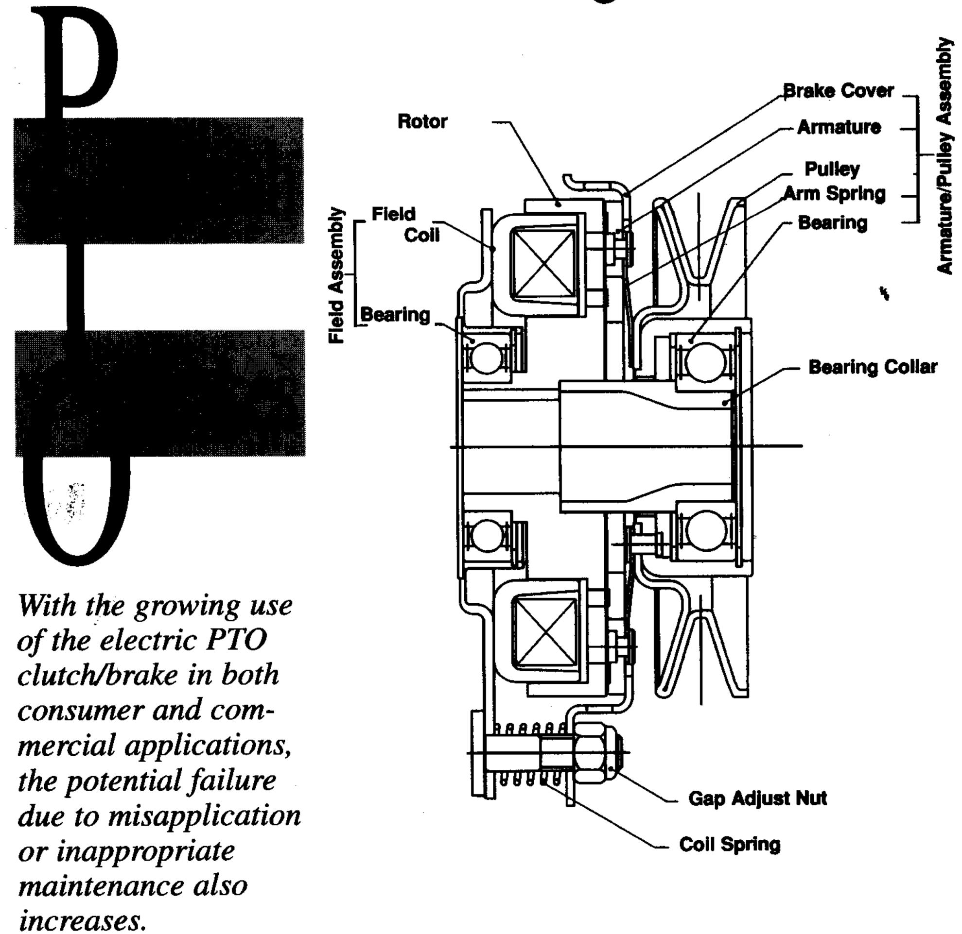
By following the steps listed below, you should arrive at the solution to the four most common customer complaints about electric clutches.
