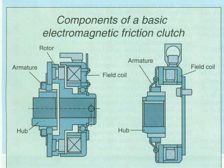
the armature against the rotor and the mating surfaces meet, producing friction. The output shaft begins spinning and quickly accelerates to match the rotor speed. A properly sized EMFC is 100% efficient, meaning it transmits all the prime mover's torque to the load. The armature and rotor essentially become one assembly after engagement, without any slippage.
