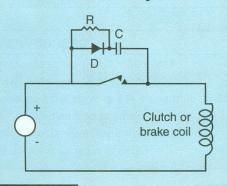
This circuit shortens decay time. When the coil is turned off, the current continues to flow and goes into the capacitor extremely fast. This is because the only resistance the current "sees" in its path is the small dc resistance of the coil and the smaller forward resistance of the diode. The value of the resistor connected in parallel with the diode is much higher than that of the diode's forward resistance so current flows into the diode and dissipates quickly.
