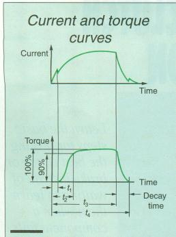
These graphs show two curves drawn to the same time scale. The curves represent clutch-torque buildup time and coil-current buildup time.
