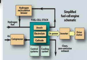
To prevent the fuel-cell anode from degrading, there must be a supply of hydrogen greater than the minimum (stoichiometric) value that the fuel-cell stack needs. This results in excess hydrogen fuel at the exit of the stack. The recirculation blower compresses and sends the unused fuel back to the inlet of the fuel cell.
