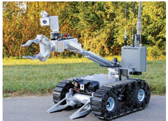
The HD1 can travel at speeds up to 4.3 mph and easily maneuvers through openings up to 26 inches wide and 31 inches high.
