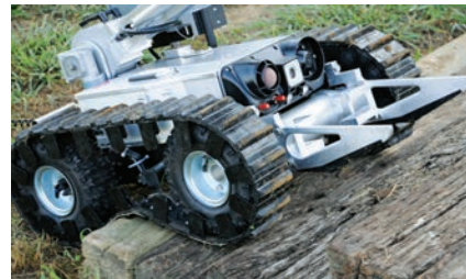
Tracked articulators make the HD capable of navigating rough terrain, climbing stairs at over 45 degrees and over objects 8 inches tall.
