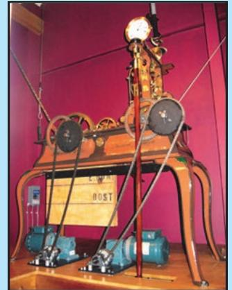
*Original clockworks with manual winding chains replaced with clutch and motor gearbox*
