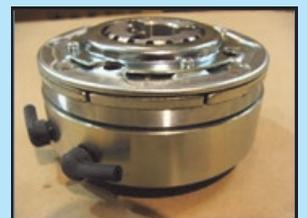
*Ogura model CT20 electromagnetic clutch*
